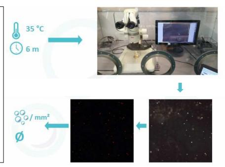
At Cristalens, the acceptability threshold is set at 100 microvacuoles per mm $^2$  and an average diameter of less than 15  $\mu$ m.
