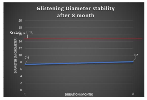
Cristalens now achieves a result at 27 days of 11 to 57 microvacuoles per mm<sup>2</sup> with a diameter between 6.7 and 8.7  $\mu$ m and a result at 6 and 8 months of 23 to 43 microvacuoles/mm<sup>2</sup> with a size between 7.6 and 9.4  $\mu$ m
