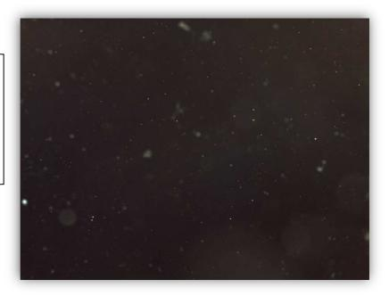
Microvacuoles form around hydrophilic microdomains<sup>1</sup>, or due to variations in the solubility of water in the polymer<sup>2</sup>.
